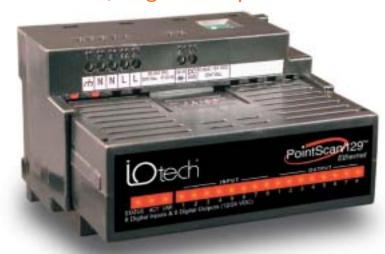
The PointScan/129 is used to monitor digital devices including proximity switches, limit switches, power circuits, and pushbuttons as well as to control relays and indicators
