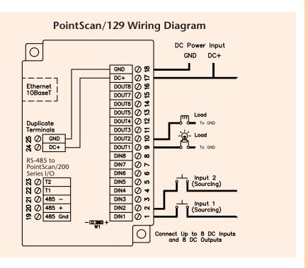
loads are switched off. They also are rated to handle the high in-rush current (5A) when switched ON. For applications where it is necessary to drive a load that exceeds the PointScan/129 module's (1A) current output rating, or when using a voltage source other than one powering the module, an interposing relay or power switch can be used.
